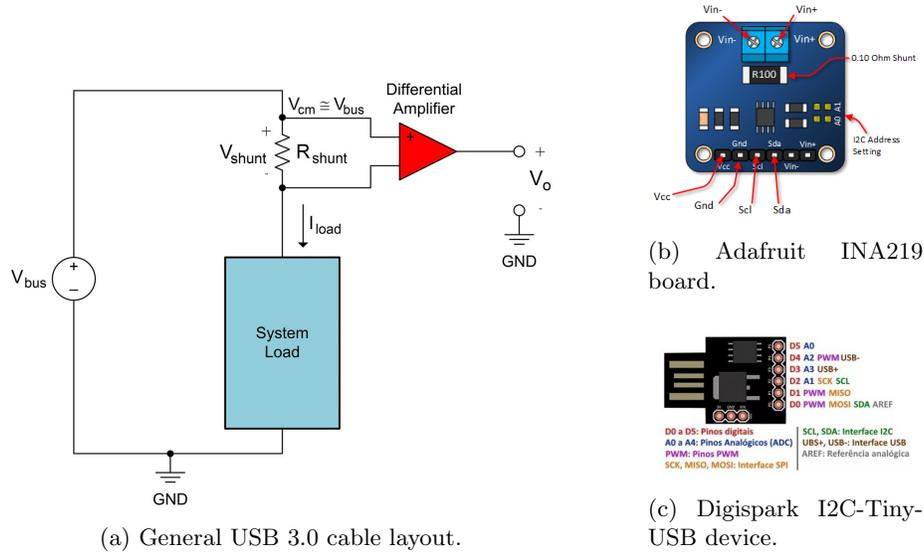
Fig. 2: Diagram of the transformed USB cable to measure consumption through the USB output, board breakout of the Adafruit INA219 board employed in our setup and I2C-Tiny-USB device.
