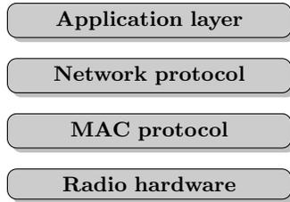
**Fig. 1.** A simple wireless sensor network protocol stack.
