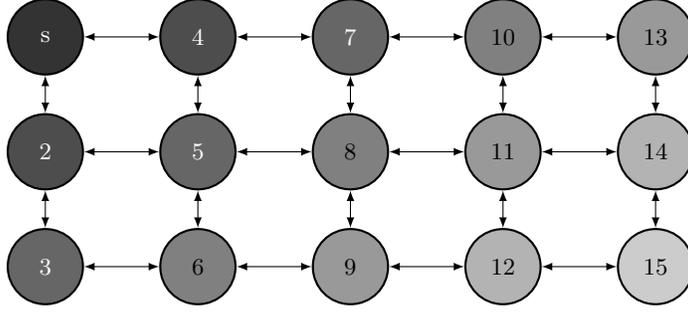
**Fig. 2.** Node ‘s’ is the sink to which all other nodes route their messages. Any two nodes that are connected by arrows can communicate. In more realistic topologies some links may only be unidirectional since radio links can be asymmetric.
